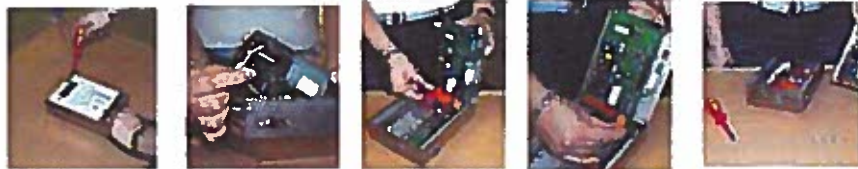
Fig. 28: Replacing a controller
