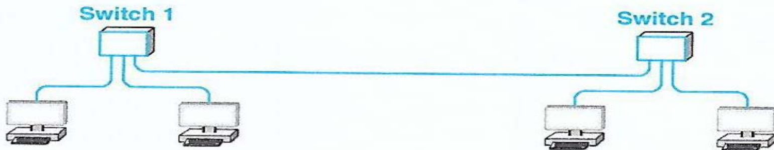
Figure 25.4 Four hosts connected by two switches.
