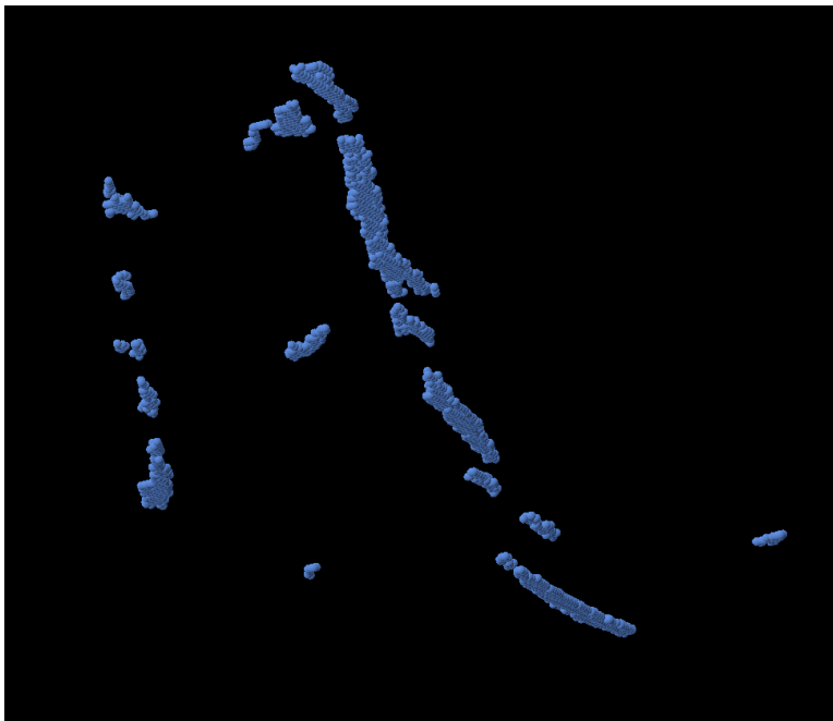
Figure 10.10: A set of points showing the salt delineation for a given seismic cross-section, but in the wrong coordinate-system, making them appear in Petrel so far away from the cube that the cube itself is not visible when looking at the points
