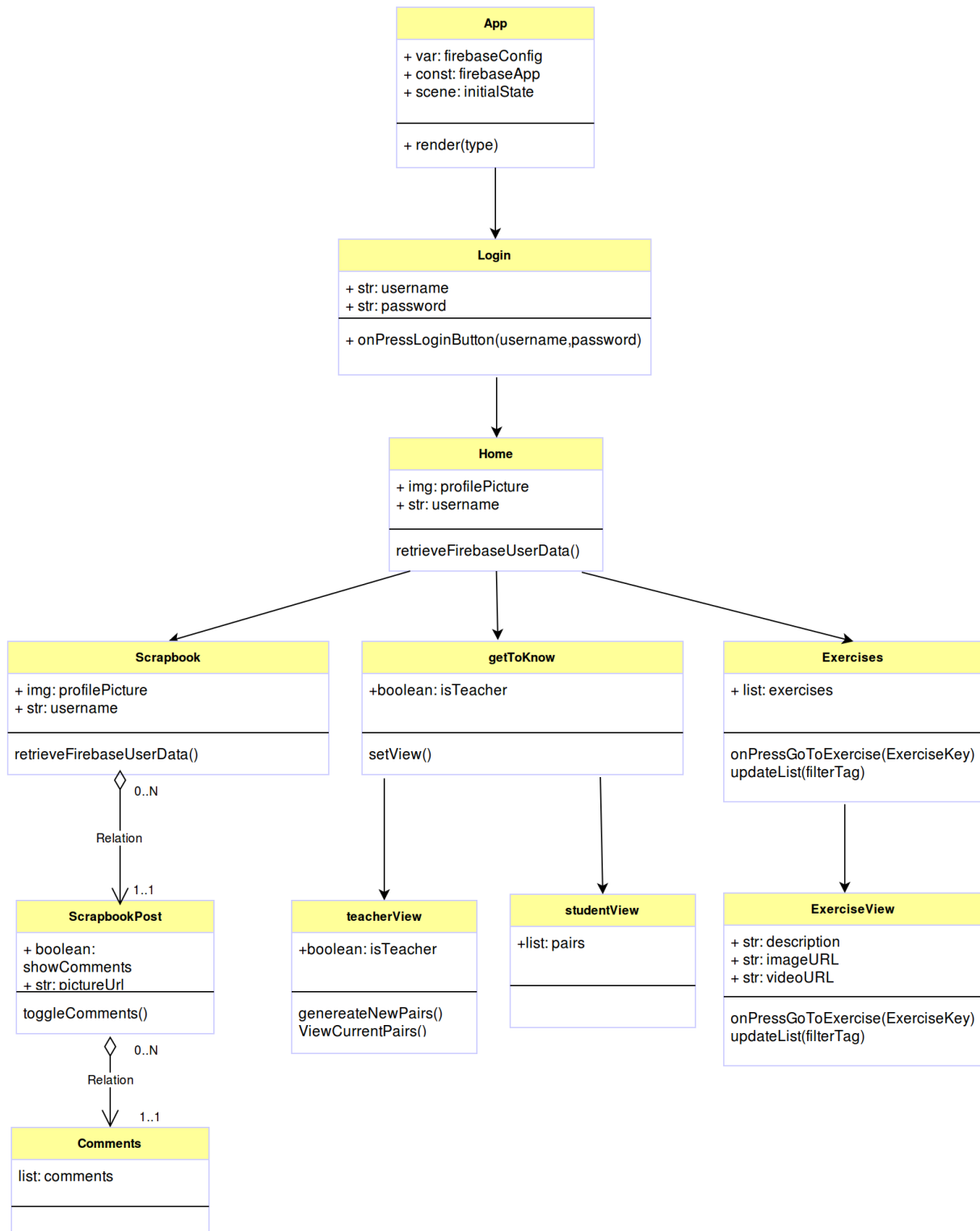
Figure 8.3.: Diagram showing the most important classes, fields and methods
