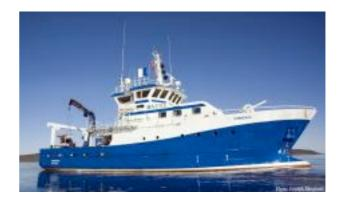
geology, archeology, oceanography and fisheries research. The ship is fitted with a dynamic positioning system and a HiPap 500 unit. This provides optimal conditions for ROV operations and the positioning of any deployed equipment. In addition to research, the ship is used for educational purposes and will become an important platform for marine courses at all levels and disciplines.
