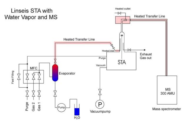
1 I water will be transferred into 1673 I water vapor at 1013 mBar
