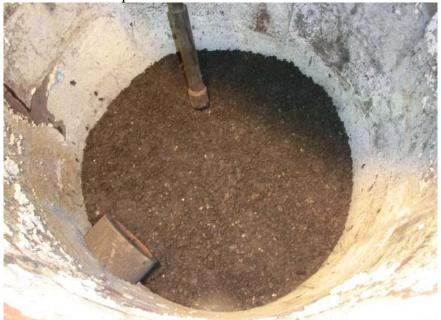
The next step is the make sure that the furnace wont leak when sand is filled in the gap between the template and the outer mantel. Finish up the lining around the tap hole, and use tape to fill all the gaps in the outer mantel and the template. Sand can now be filled in the
