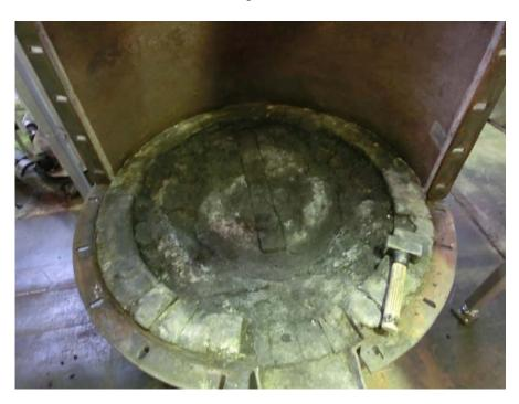
Apply coal tar to the bottom of the furnace to ensure contact between the bottom electrode and lining (probably not strictly necessary).
