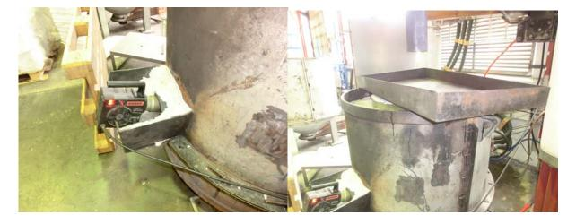
Even after drying the lining will contain moisture and the area around the tap hole can be dried with a propane burner.
