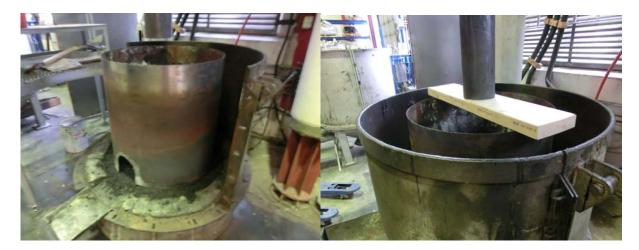
Use a carbon crucible as a tapping hole. Around 7cm of the crucible should be inside the furnace. A thin layer of coke (Around 2 cm) is place in the bottom of the furnace, inside the template. This should make the inner part of the furnace easier to remove after the experiment.
