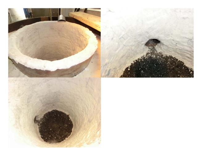
Cover the top of the furnace and use some kind of heating device to dry and harden the lining 48 hours or more.
