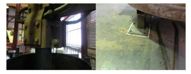
The template for the inner lining can now be placed inside the furnace. Centre the template inside the furnace, and centre the furnace under the electrode. The front of the furnace can now be put in place and secured with bolts. The electrode can be used to hold the template in position for the next steps.
