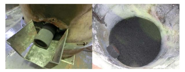
Alumina lining paste is now used to hod the tap hole crucible in place.
