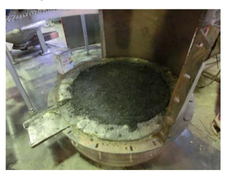
It is convenient to now put the electrode in the electrode holder. Make sure that the electrode is long enough, and not how much the electrode can be moved up and down during the experiment. The electrode height must probably be adjusted by moving it up or down in the electrode holder after the furnace has been built. Remember to place the plastic feet under the furnace.
