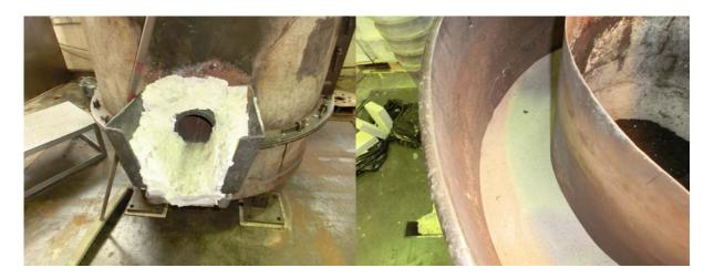
When the sand has been filled the electrode can be raised as the template is held in place by the sand. The inner lining can now be built. Cut the lining into manageable pieces, and use a hammer to compress the lining. Two layers of lining (a total of approx 7cm) are used in the bottom 30 cm of the furnace.
