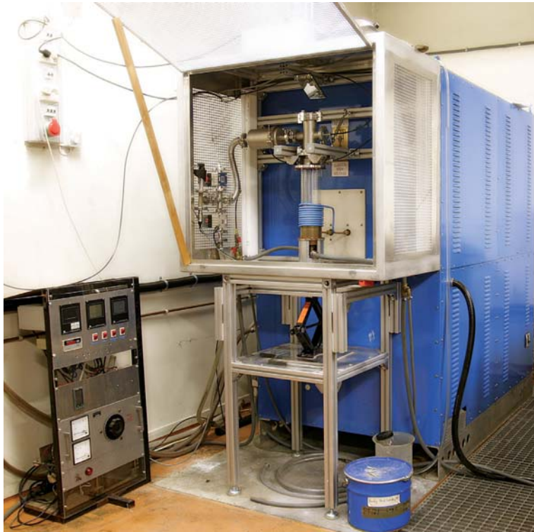
Figure 3.3: Picture showing the cold crucible induction furnace ©Melinda Gaal
