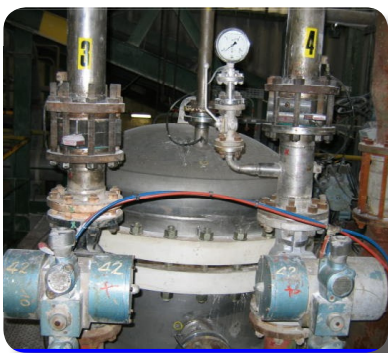
Chemical Reactor fitted with sensors (BARPI)
