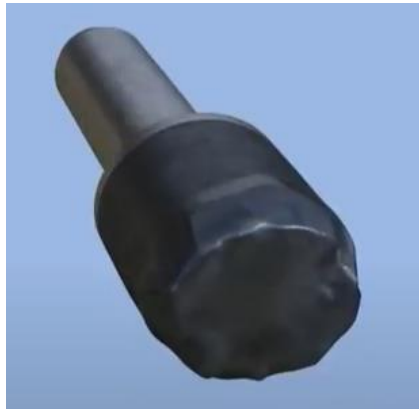
Plug head erosion
