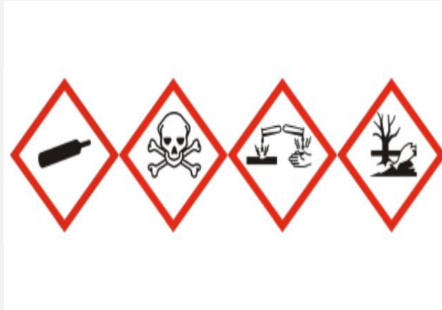
Hazard labels for Ammonia
