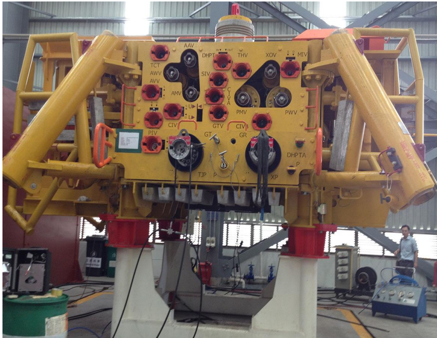
Electro-hydraulic tree by One Subsea
