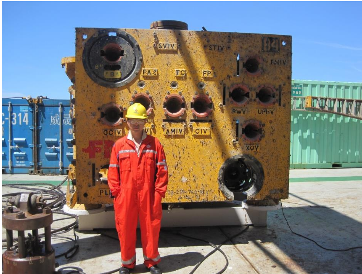
Subsea hydraulic tree in Liuhua 11-1 oil
