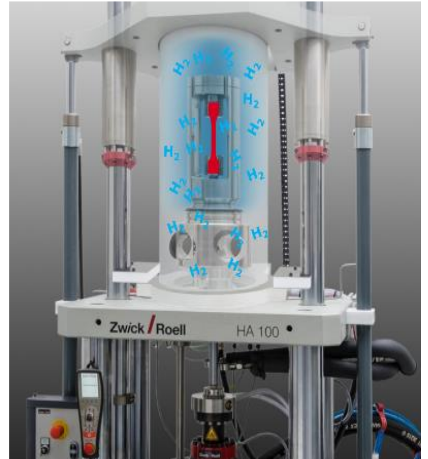
High Pressure Autoclave [Adapted from MPA Stuttgart]
