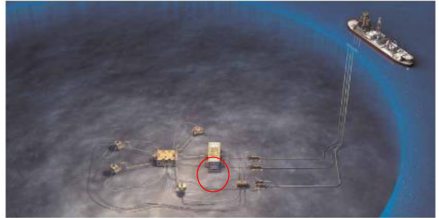
Fig. Typical subsea field layout with wells connected to a central manifold, a pump station (in red) and a topside facility
