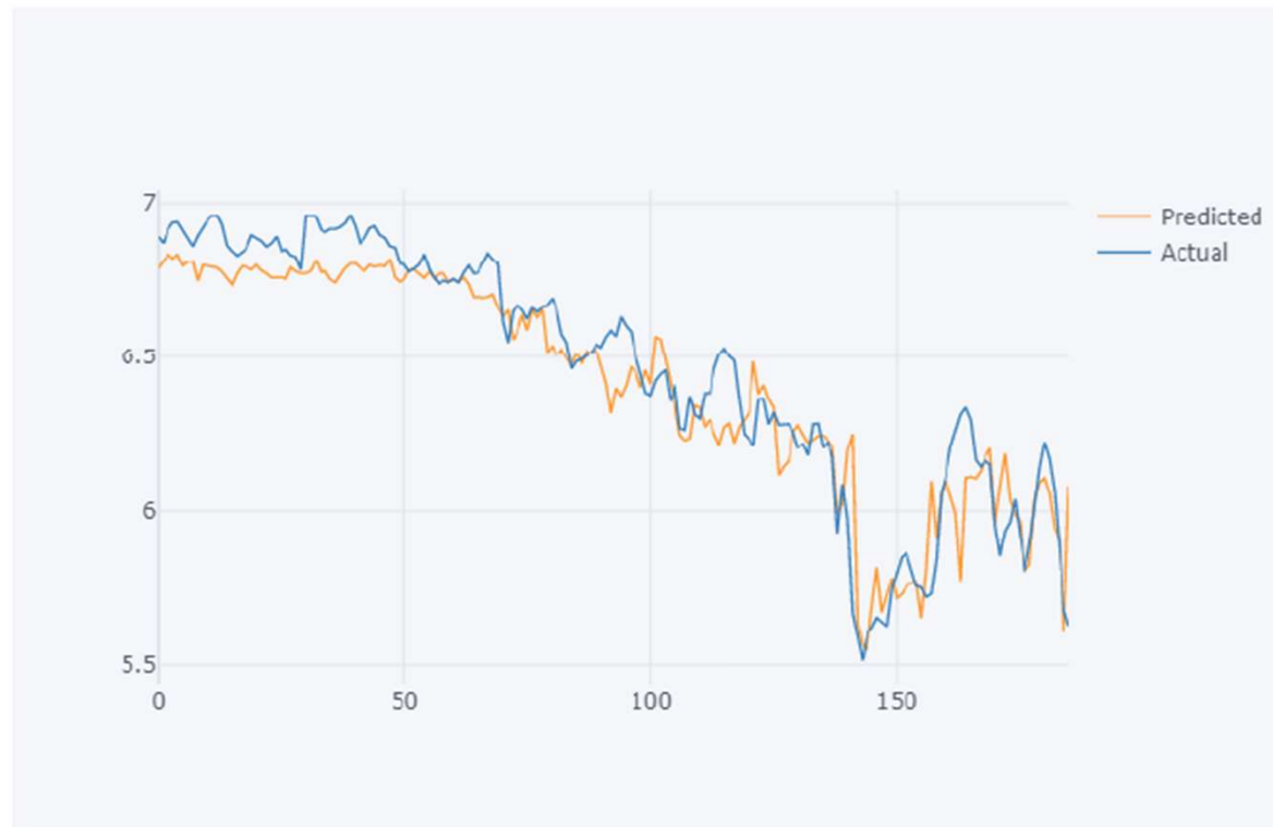
Figure 6.4: Example of the predictions of the 4-layered LSTM model for 7 days ahead prediction, compared to the actual flow values. Illustrated on one of the degrading flexibles
