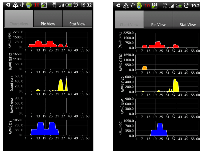
Figure 19: Power usage with business logic on client (left) and business logic on sever (right). Test Client Provided by the TABuss project.
