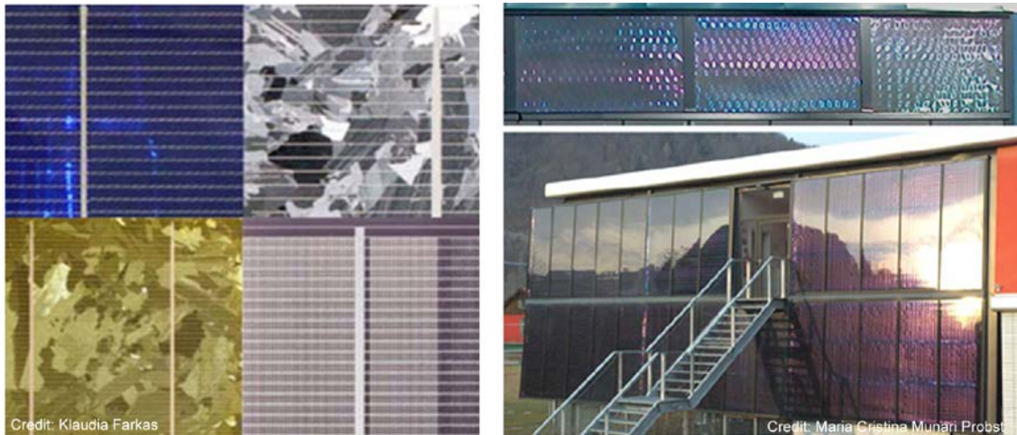
FIG 7.4: (Left) Range of colours in PV; (Right) visible colours due to the sunlight striking onto the extra white glass above the absorber of STC system,
