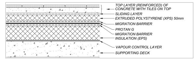
In cases of insulation on the «wet» side of the waterproofing membrane, make sure a non water absorbing insulation is used (eg. extruded polystyrene, XPS). Protan G 1,5mm can normally not be mechanically fastened to withstand wind loads.
