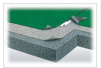
Protan GT 2,4mm is installed on the horizontal surfaces. Details and terminations are executed with Protan GT 1,4mm.
