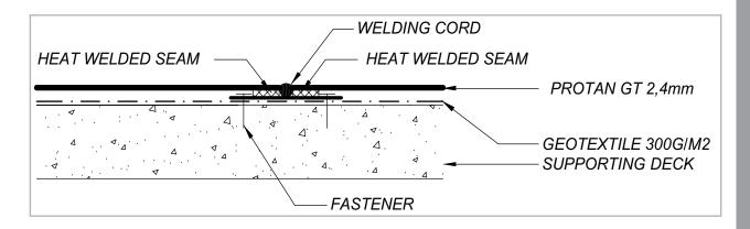
The finished result depends largely on the substrate. Protan GT is dimensionally stable - thus the best result is achieved by installing on dimensionally stable substrate for example smooth concrete deck.
