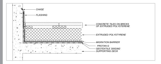
Protan G 1,5mm has hot air welded seams and is loosely installed, either on un-insulated or insulated supporting decks. On insulated decks it can be installed
