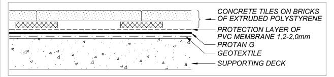
A protective layer over the membrane is needed to prevent mechanical damage or negative chemical influence. The membrane is UV resistant and needs no additional protection on vertical details directly exposed to sunlight.
