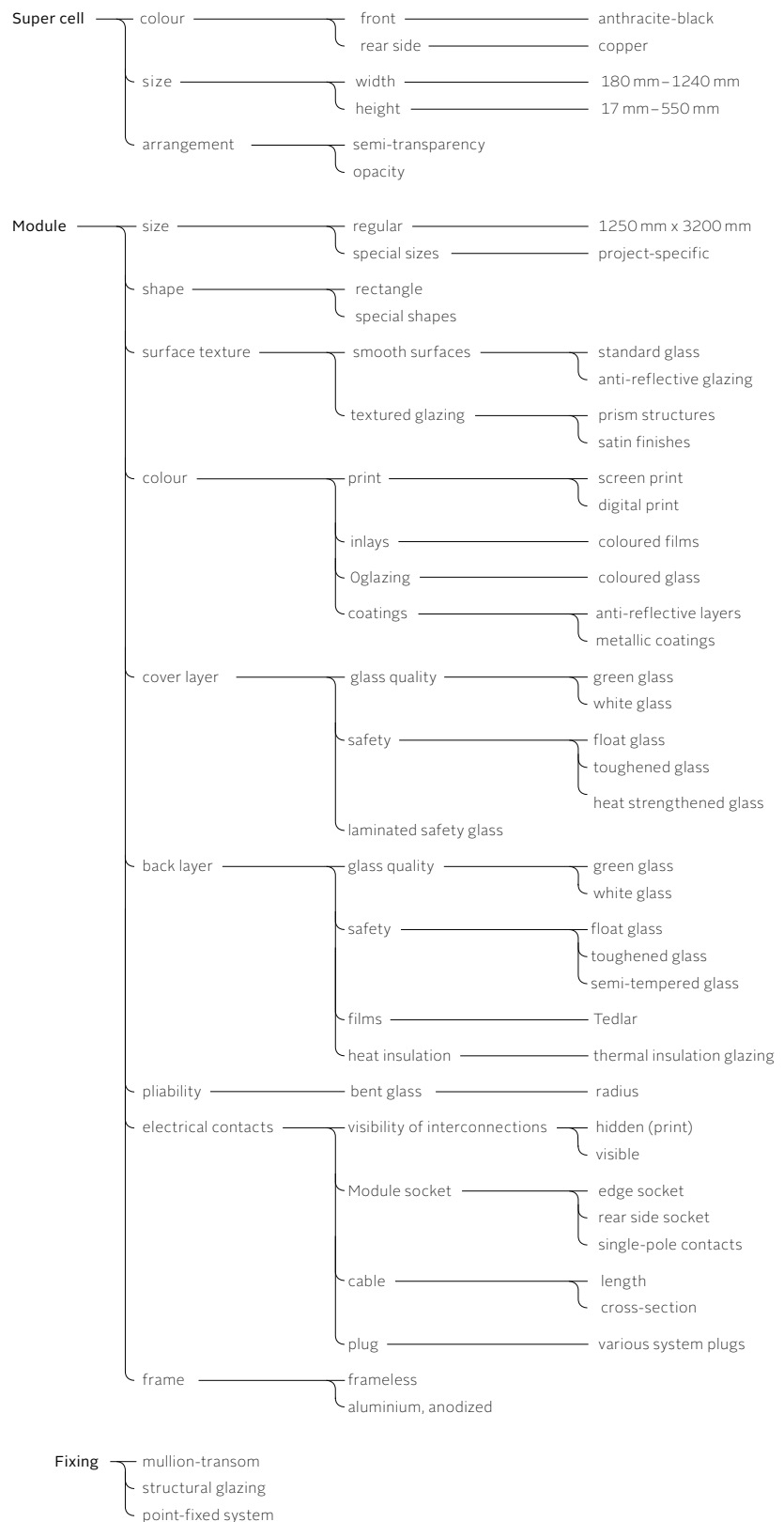
Fig.30 Solar module design options, using Odersun AG products as an example
