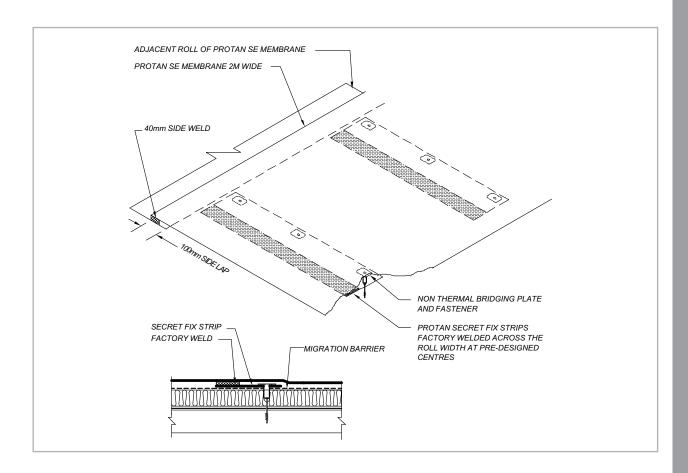
This system minimises the on-site fabrication with the advantage of being able to install 2m wide membranes in all zones of the roofing surface, thus increasing the installation speed. The strips have higher pull out value than the regular Protan SE membrane, which makes it a good alternative to the Standard Overlap System in areas of high wind design value.
