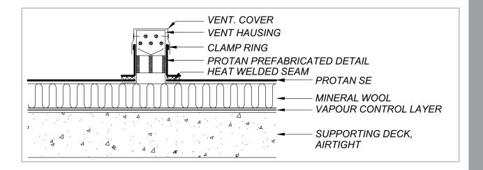
A correctly designed and installed vacuum roof «sucks» itself firmly to the substrate.
