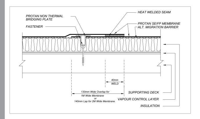
Mechanical fixings and tube washers should be fixed within the laps at appropriate centres, in accordance with local wind standards. The fixings are placed on premarked lines at a distance of minimum 30mm in from the longitudinal edge.
