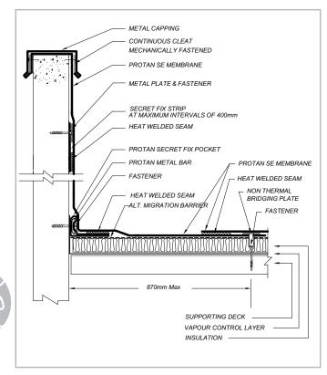
Protan Exposed Membrane Roof
