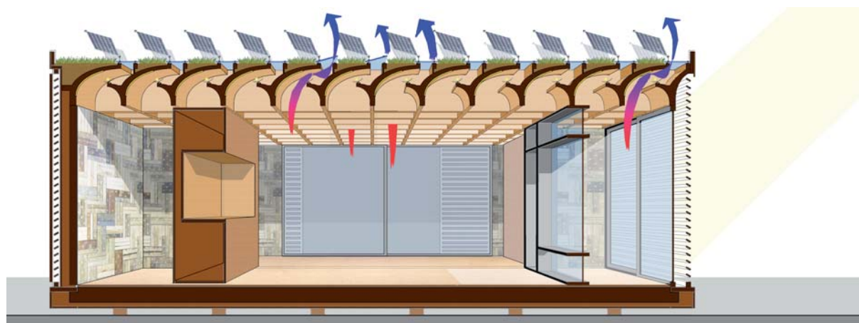
Fig. 5 - Section of the ZE+hytte: permeability of the roof, buffer spaces and solar protection.
