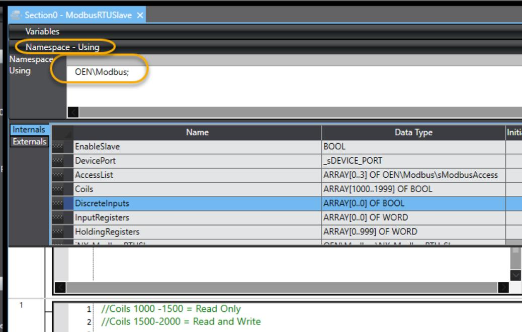
The screenshot shows a software interface with a 'Variables' section. Under 'Namespace - Using', the text 'OEN\Modbus;' is entered and highlighted with a yellow circle. Below this is a table with columns 'Name' and 'Data Type'. The table lists several variables:
