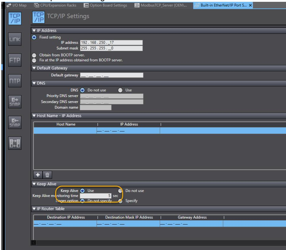
When using “Keep alive” the TCP socket will send a keep alive message to the client, to check if the client is still responding. If the client does not respond within the “Keep Alive monitoring time” the socket will close, and reopen for new connection for the client.
