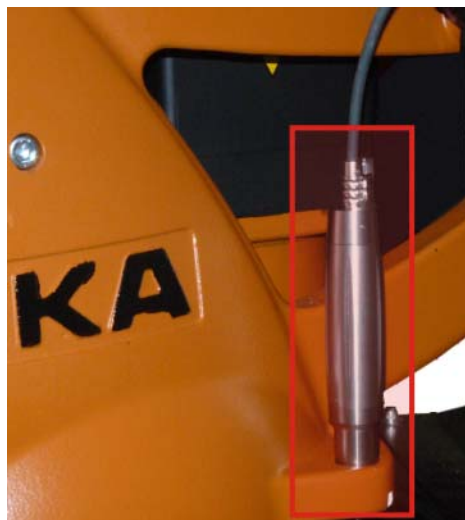
Fig. 3-2: EMD in operation
