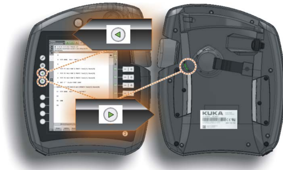
Fig. 4-9: Program execution directions: forwards/backwards
