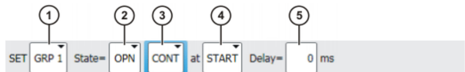
Fig. 9-3: Inline form for gripper with approximate positioning
