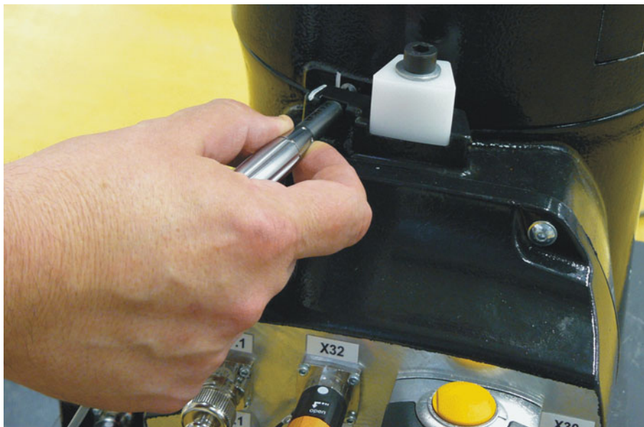
Fig. 5-16: Screwing MEMD onto gauge cartridge
