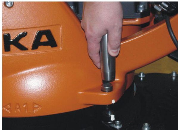
Fig. 5-7: Removing protective cap from gauge cartridge
