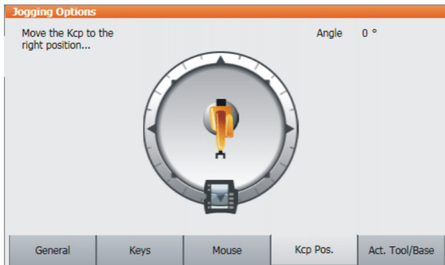
Fig. 4-22: Defining the alignment of the Space Mouse
