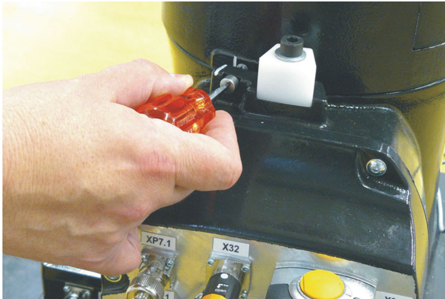
Fig. 5-15: Removing protective cap from gauge cartridge
