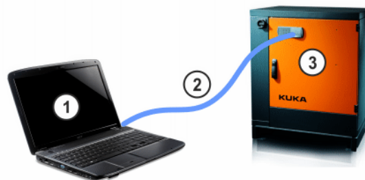
Fig. 7-1: Example: connection between WorkVisual PC and robot controller
