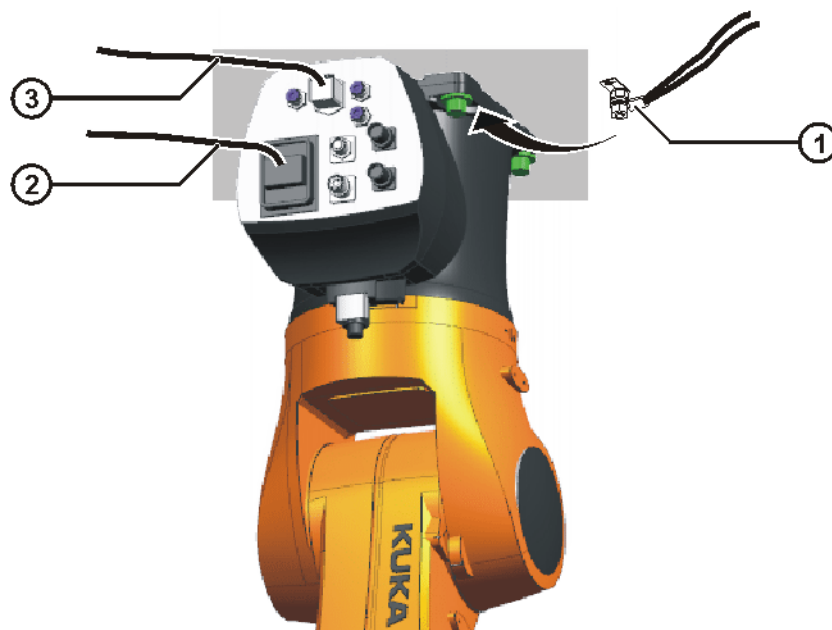
Fig. 8-15: Connecting the cables
