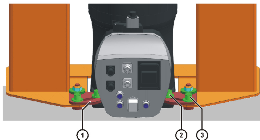
Fig. 8-5: Positioning and fastening the swivel holders
