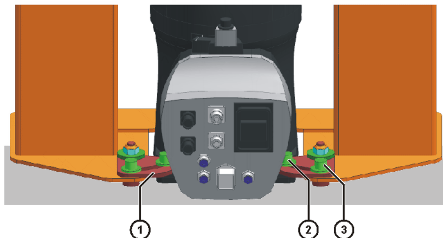
Fig. 8-11: Positioning and fastening the swivel holders
