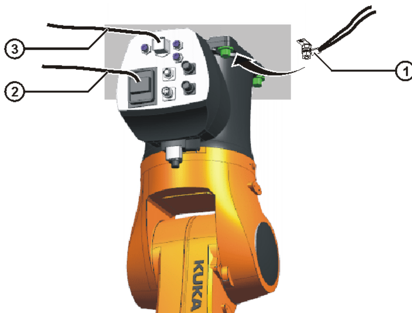
Fig. 8-15: Connecting the cables
