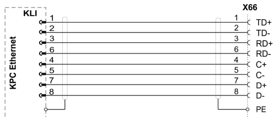
Fig. 6-11: Connector pin allocation X66
