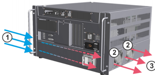
Fig. 3-11: Cooling circuit, drive box
