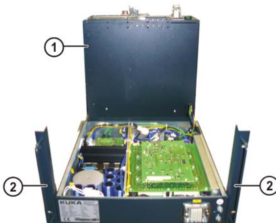
Fig. 11-3: Drive box and control box separated
