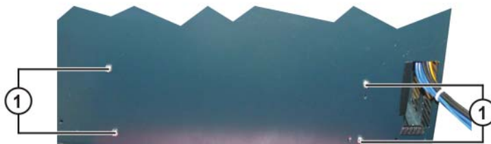
Fig. 11-15: Low-voltage power supply unit, fastening
