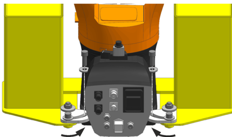
Fig. 6-3: Fastening the base frame of the Load Lifting Attachment (rear of robot)
