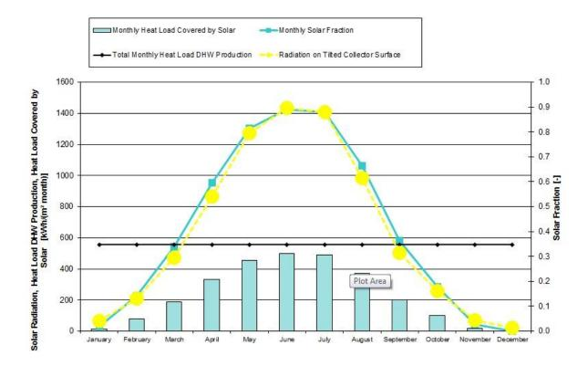
The figure above shows that there is a huge gap between the heat load covered by solar thermal collector and the heat load DHW energy production in the winter. This means that during winter, most of the DHW heating will be provided by the heat pump.
