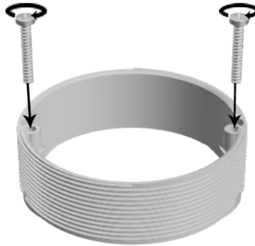
Figure 1.3: Inserting screws into adjustment rings
