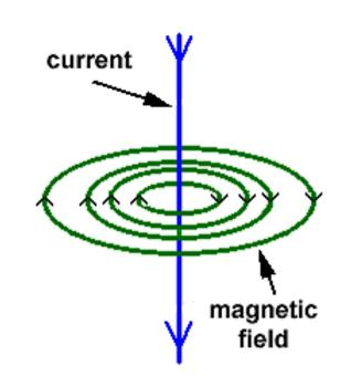
In magnetostatic, such as constant DC current,  $\frac{\partial D}{\partial t} = 0$
