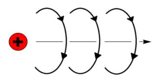
Magnetic field in vacuum generated by moving charge q:
