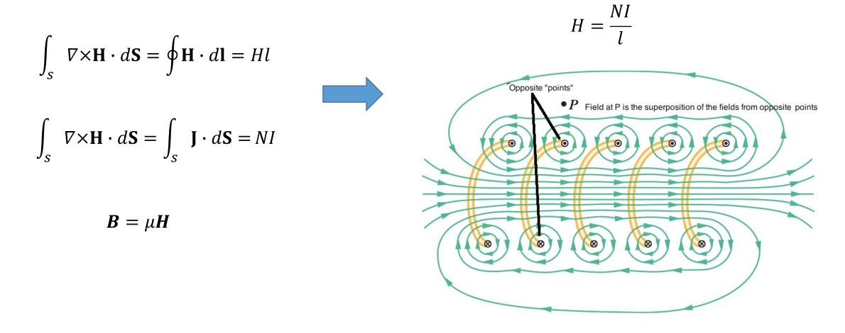
If the core is iron instead of air, the flux density **B** is much stronger.
