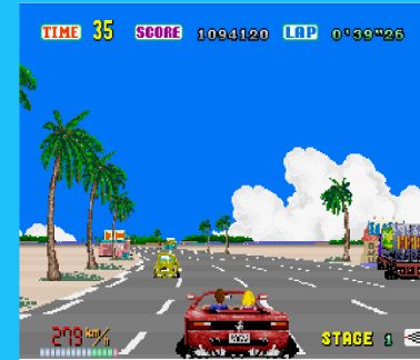
Figure 30 Fake 3D in the game Outrun (1986). The sprites of the palm trees and cars are scaled depending on their distance and drawn from back to front. Parallax scrolling is used for the clouds in the back, and the road is drawn with geometric primitives.
