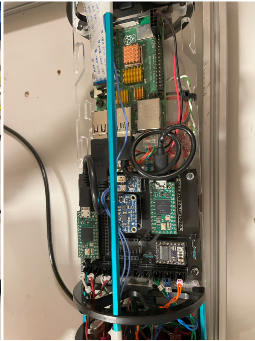
(b) Picture of new electronics. Note: Second motor and driver is not connected on this picture.
