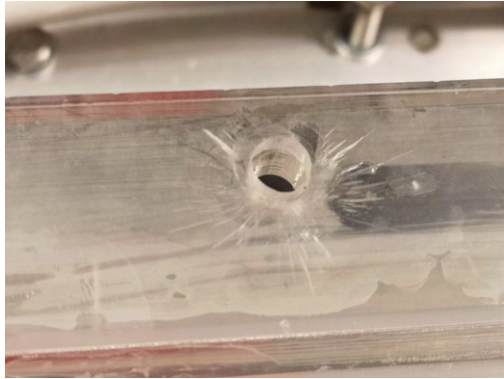
Figure 3.29: Cracks, 4mm plates.
