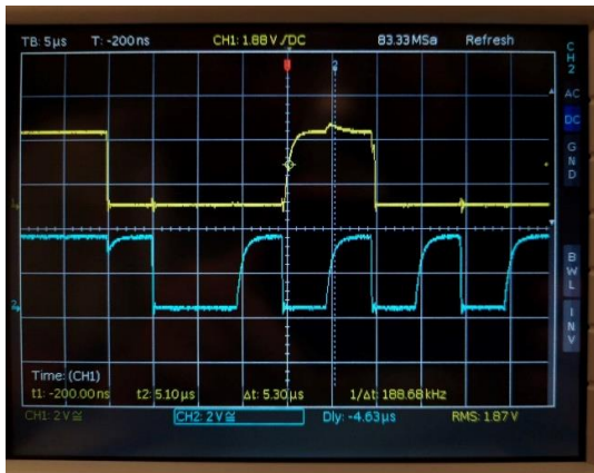
Figure 1 - I2C over 3m cable WITHOUT bus buffer.
