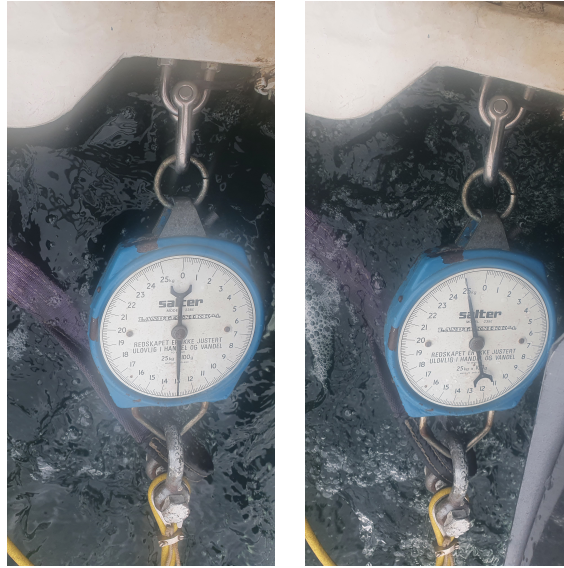
Figure 5.50: Left: Drag force from ROV at 1.3 m/s Right: Drag force from ROV at 1.7 m/s
