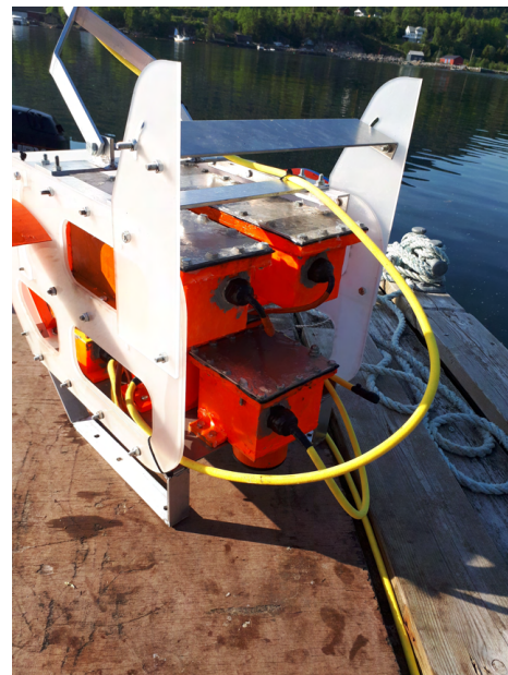
Figure 4.40: Boxes with equipment placed in ROV
