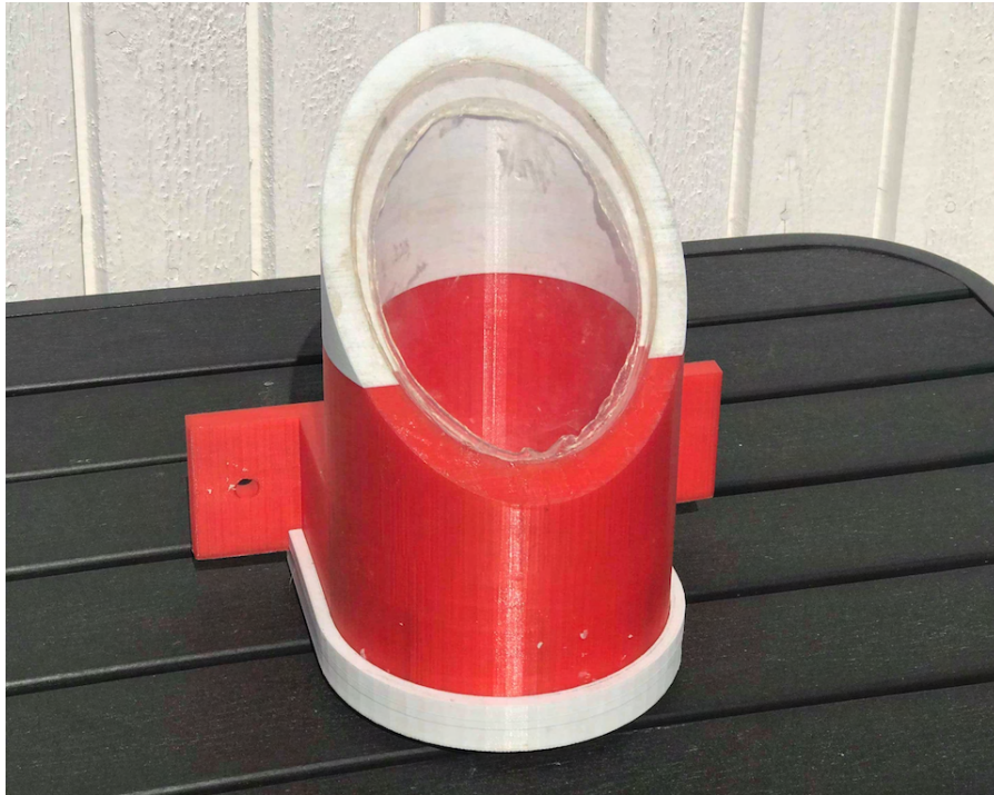
Figure 4.8: 3D printed camera housing
