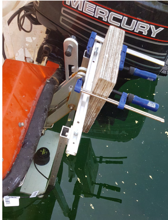
Figure 4.42: Mounting echo sounder to boat
