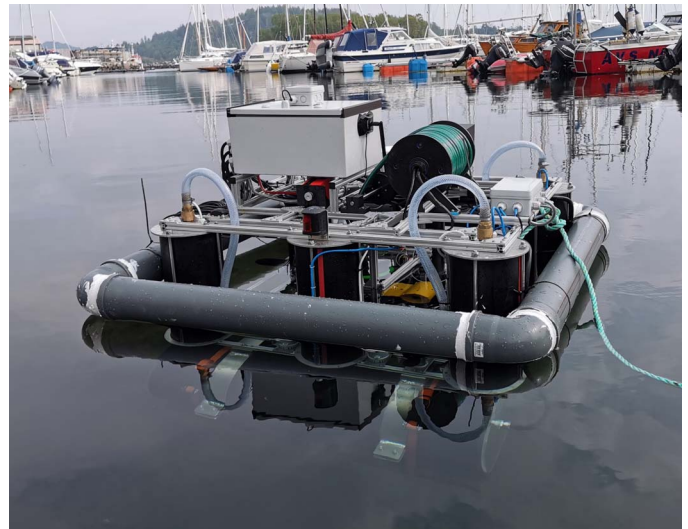
Fig. 4. "Sea Farm Inspector Platform with "lifebuoy" due to stability issues.
