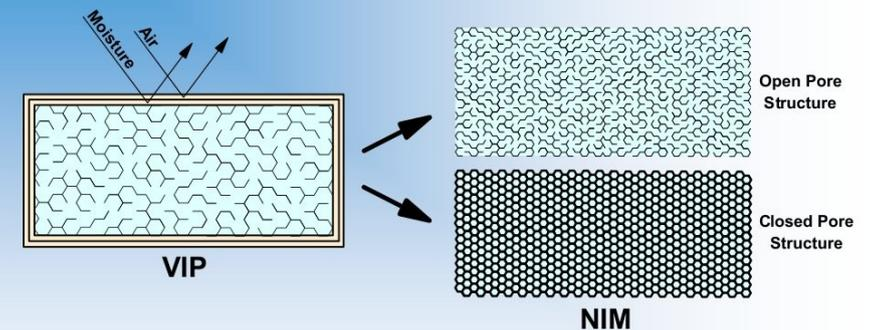
NIM - A basically homogeneous material with a closed or open small nano pore structure with an overall thermal conductivity of less than 4 mW/(mK) in the pristine condition
