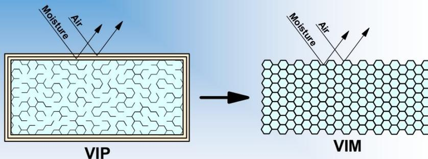
VIM - A basically homogeneous material with a closed small pore structure filled with vacuum with an overall thermal conductivity of less than 4 mW/(mK) in the pristine condition
