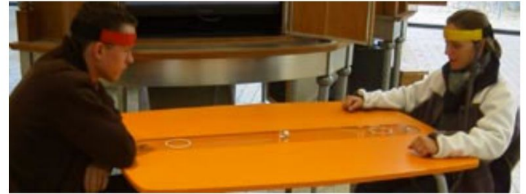
Fig. 2. Brainball: players' EEG signals control the movement of a physical ball on a table.
