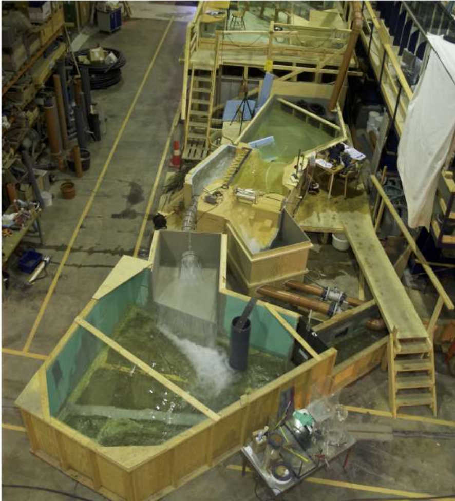
Figure 2-1: Physical model of closed conduit spillway at Storlivatn (photo taken from Baard Aasmund Utvik Gjerde's master thesis)
