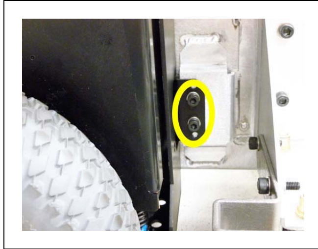
Figure 8-13. Mounting Screws at Bottom-Right of Drive Assembly
