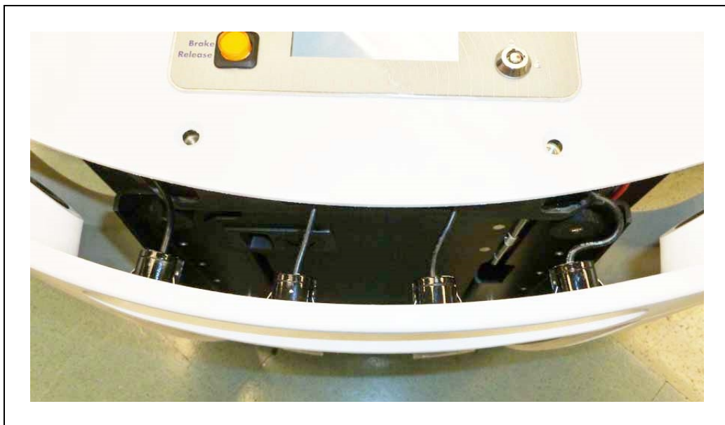
Figure 8-18. Sonar Leads, with Connectors Still in Chassis
