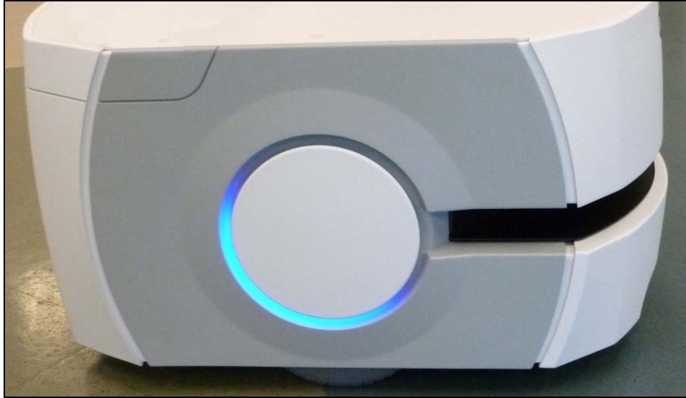
Figure 8-20. Right Side Skin, Showing Even Gaps at Edges
