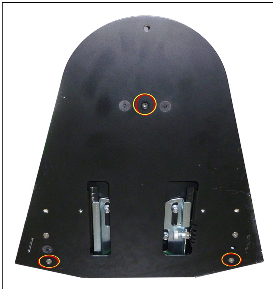
Figure 3-18. Underside of Docking Station Foot, Showing Screw Locations
