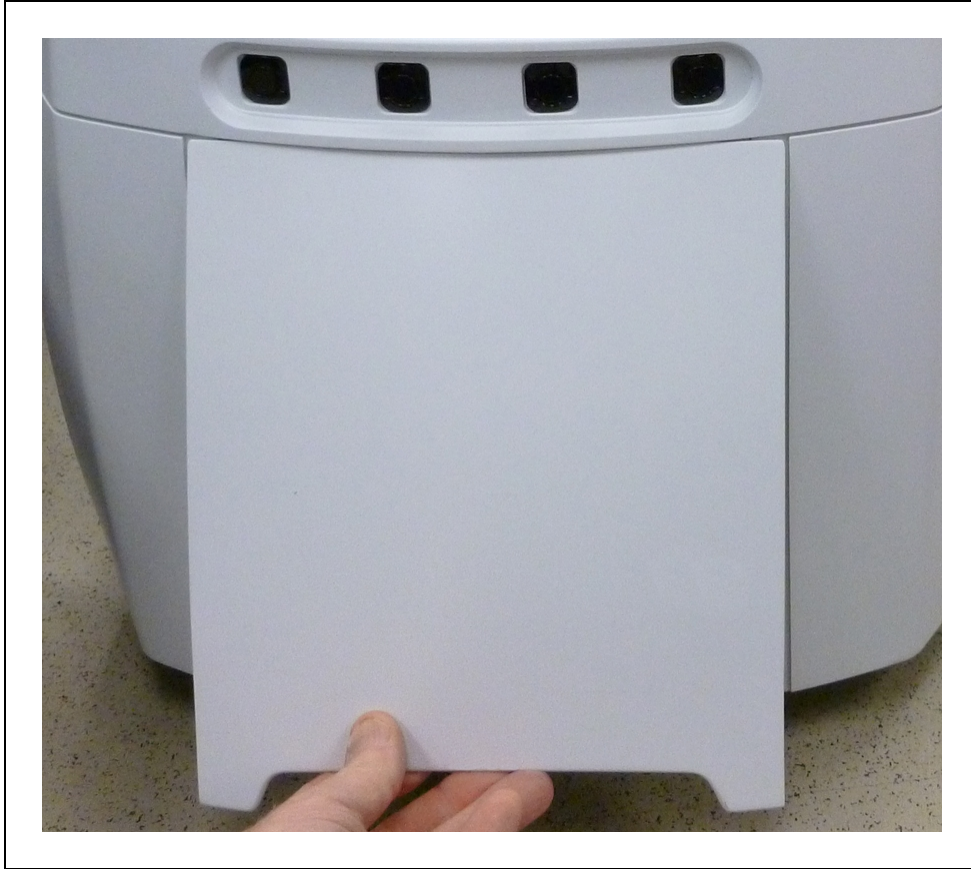
Figure 3-10. Pulling the Bottom of the Rear Platform Cover Out
