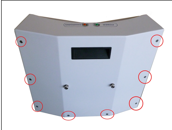
Figure 8-9. Docking Station Rear Cover Screws (8 of 10)
