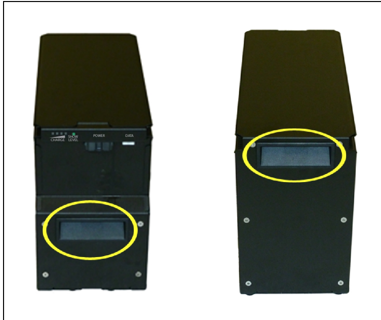
Figure 8-4. Battery Recesses, for Gripping
