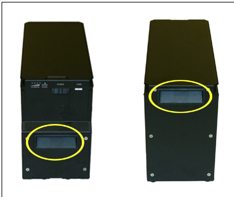
Figure 3-12. Battery Recesses, for Gripping
