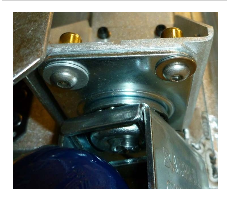
Figure 8-15. Rear Caster, Two Screws and Washers
