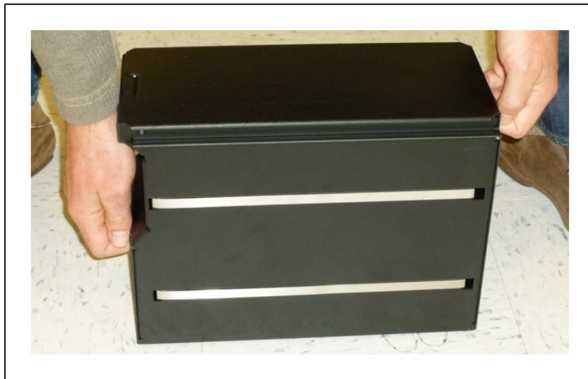
Figure 2-7. Lifting the Battery
