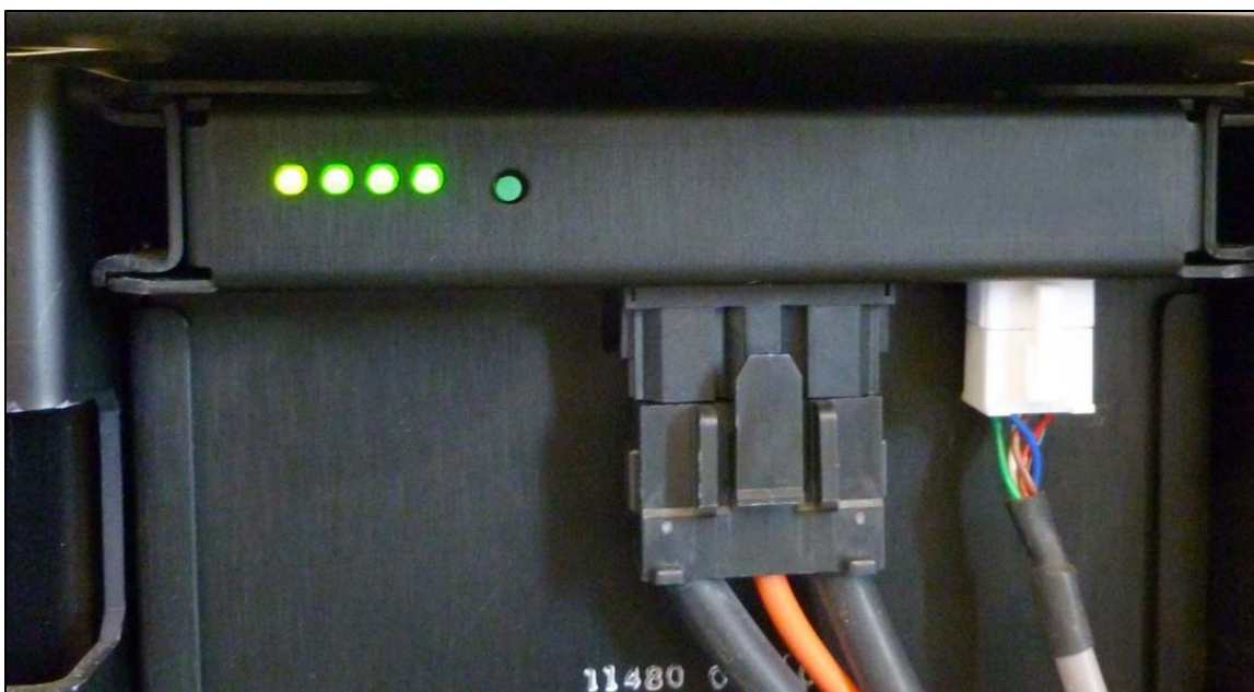
Figure 4-1. Battery LEDs, Push-Button, Power Cable, and Data Cable
