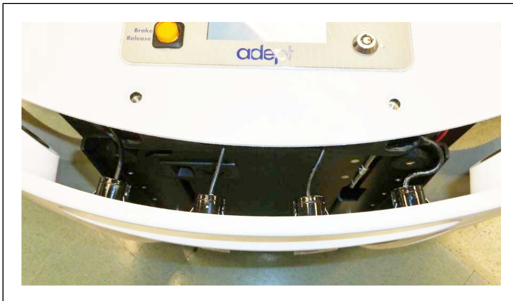
Figure 8-2. Sonar Leads, with Connectors Still in Chassis
