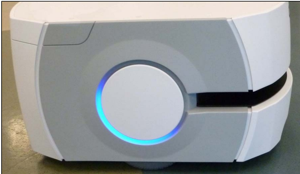
Figure 8-4. Right Side Cover, Showing Even Gaps at Edges
