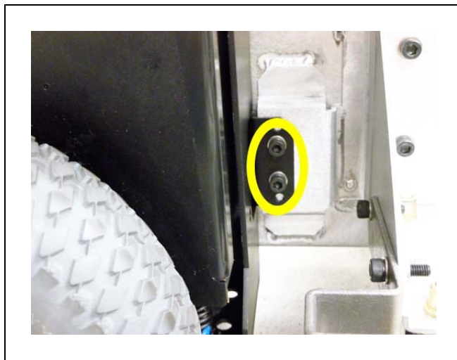
Figure 8-14. Mounting Screws at Bottom-Right of Drive Assembly
