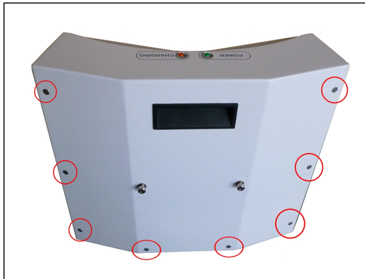
Figure 8-11. Charging Station Rear Cover Screws (8 of 10)
