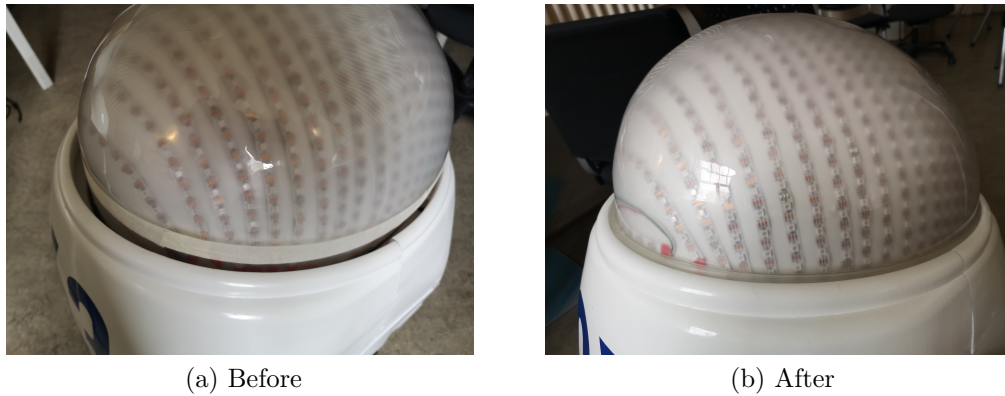
Figure 12.3: Sealing strip mounted on the LED dome.
