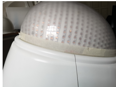
Figure 12.2: Masking tape is used to line up the sealing strip on the LED dome.
