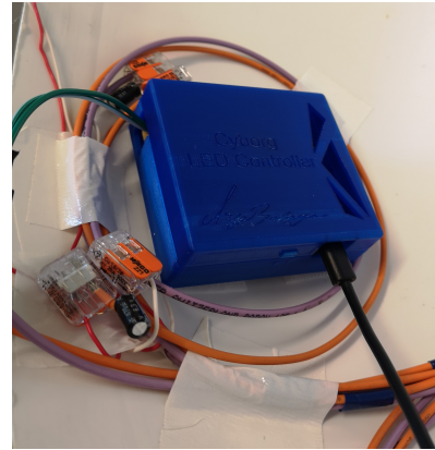
Figure 12.5: The LED controller mounted inside the LED dome with velcro tape.
