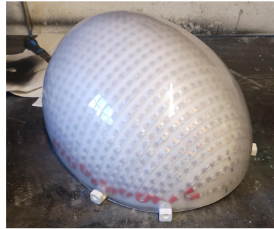
Figure 4.1: Preparing the LED dome and outer shell for the dome fasteners.
