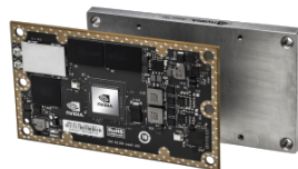
Figure 2.4: The NVIDIA Jetson TX1 module with protective case. From the NVIDIA Blog, link below.
