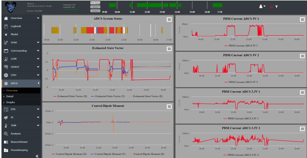
Fig. 5 Attitude Determination and Control System (ADCS) Page in the OPS Interface.
