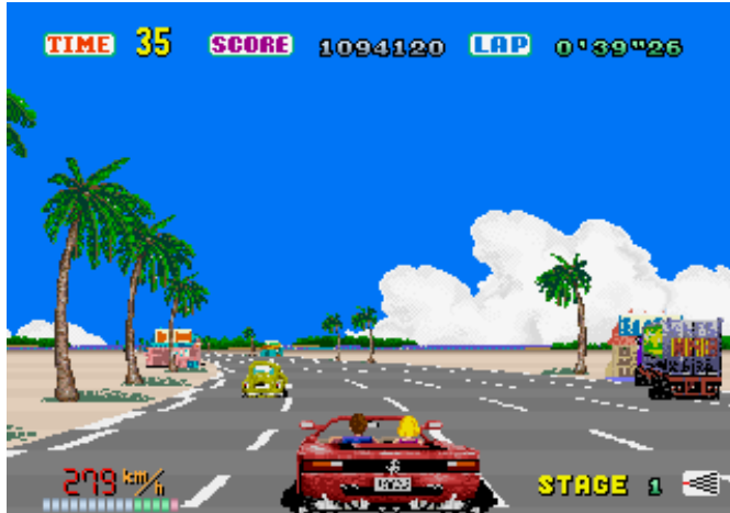
Figure 30 Fake 3D in the game Outrun (1986). The sprites of the palm trees and cars are scaled depending on their distance and drawn from back to front. Parallax scrolling is used for the clouds in the back, and the road is drawn with geometric primitives.
