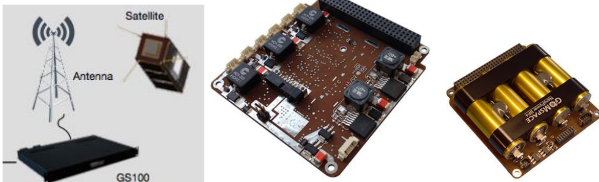
Fig. 2: Left – Ground station setup. Middle – EPS. Right – Battery package
