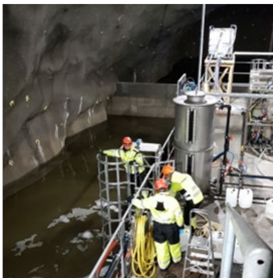
Sampling from a sedimentation basin at Bjørnegårdtunnelen (Sandvika)
